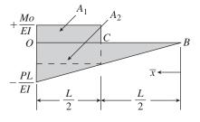
NOTE:  $A_1$  is the *M/EI* diagram for  $M_0$ (rectangle).  $A_2$  is the *M*/*EI* diagram for *P* (triangle).
