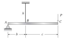
P = 240 lb b = 20 in. c = 30 in. h = 20 in.Beam:  $EI = 36 \times 10^6 \text{ lb-in.}^2$ Wire:  $EA = 1500 \times 10^3 \text{ lb}$
