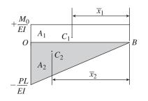
NOTE:  $A_1$  is the *M/EI* diagram for  $M_0$  (rectangle).  $A_2$  is the *M/EI* diagram for *P* (triangle).
